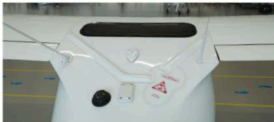
BPRS installation: hatch and belt positioning
