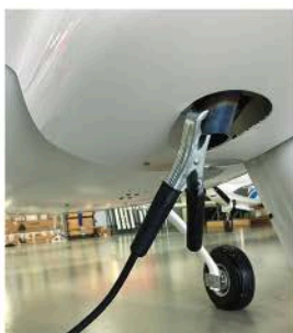
Ground wire connected to exhaust.
