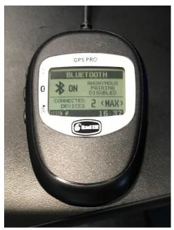
If you want to track position on iPad using ForeFlight or other EFB, connect to "Bad Elf Pro" via Bluetooth. Redbird can connect to a max of two devices at one time. If you see "2 <MAX>" displayed on Bad Elf and your device isn't connected, look for somebody close by with Bluetooth on that is connected and ask them to disconnect!
