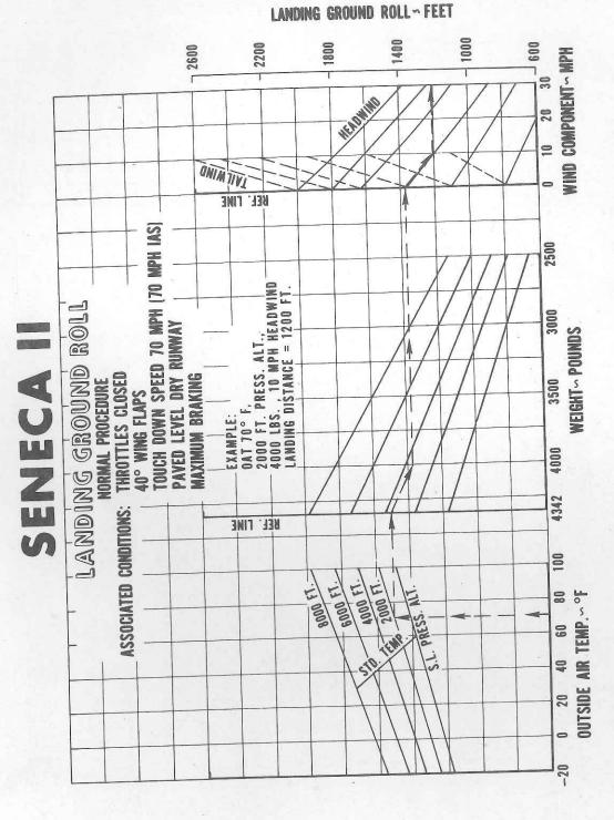
"The above distances may be reduced by approximately 25% when the aircraft is equipped with optional Heavy Duty Wheels, Tires and Brakes. (Reference Aircraft Equipment List in Weight and Balance Section of this manual.)"
